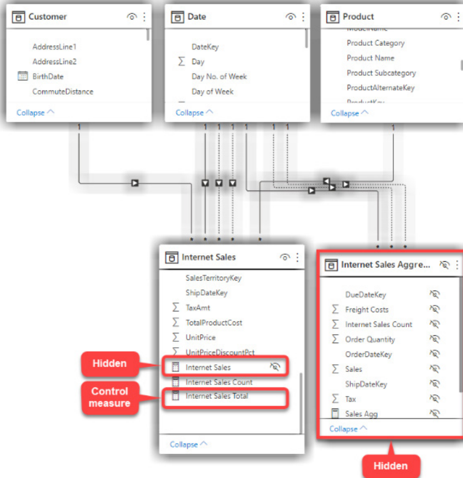
Figure 10.4 – The data model after hiding the Internet Sales Aggregated table and the Internet Sales measure
